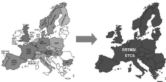
FIGURE 1: Europes challenge is to substitute more than 20 signaling and ATP systems by just one single system, ETCS, in order to provide border crossing interstate rail transit in all over the European Union.
